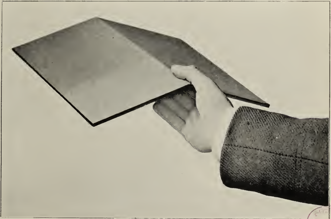
FIG 72. ALLEGED FAULTY BESSEMER PLATE, 1875
